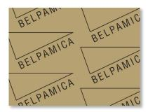
BELPA® MICA for high temperatures is made of shelly Mica compressed in sheets reinforced with perforated stainless steel 316 without binder. This material is suitable at high temperatures gaskets at low pressures and specially designed for services where high temperatures combined with fluids could promote the oxidising process of materials such as graphite.
