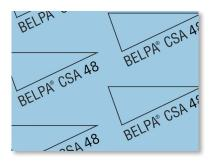
Compressed sheets for gasket made of mineral fibre, aramide and dispersed inorganic loads mixed in a matrix of type NBR rubber. The material is a sheet for gaskets for a wide range of applications. Its high compressibility, chemical resistance and good permeability make the BELPA CSA-48 suitable for most common uses, (water, air, oils, solvents, etc). It is also available with steel wire reinforcement and anti-stick coating. REF. BELPA CSA-48 M.
