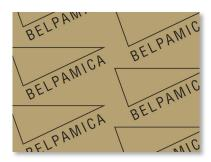
BELPA® MICA for high temperatures is made of shelly Mica compressed in sheets reinforced with perforated stainless steel 316 without binder. This material is suitable at high temperatures gaskets at low pressures and specially designed for services where high temperatures combined with fluids could promote the oxidising process of materials such as graphite.
